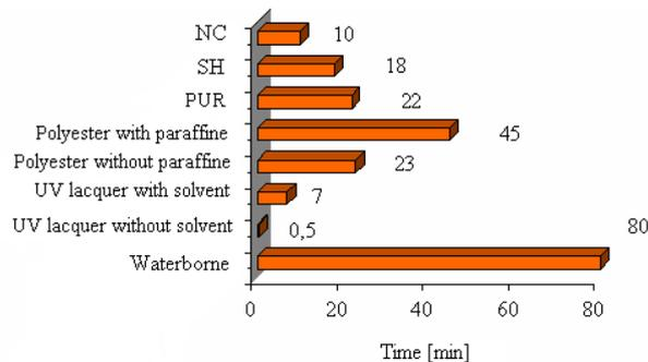
Fig. 2. Comparison of dryings time of coatings from selected lacquer products [6]
