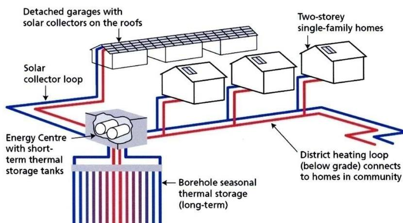
Fig. 2. Collection and storage of solar energy.
