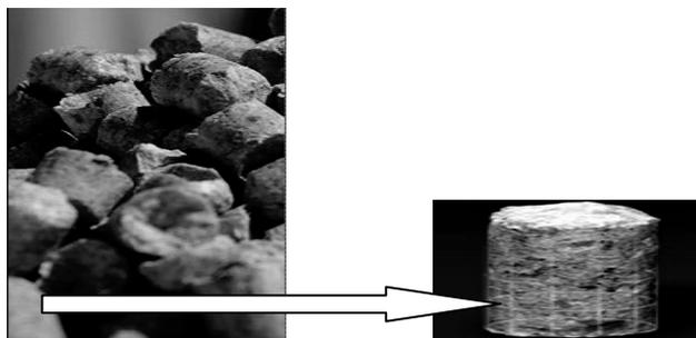
Fig. 1. Pellet mass and a single pellet
