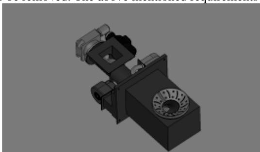
Fig. 2. The retort burner with flame modulation for the combustion of pellets or cereal grain
