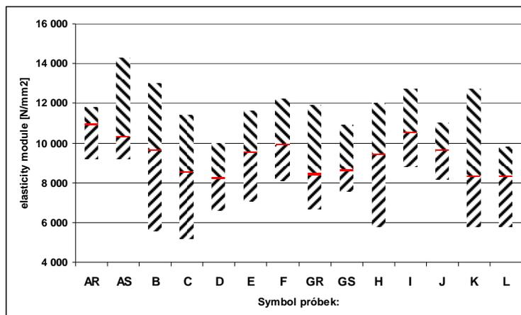
Figure 3. Characteristic values of the modulus of elasticity at 12% moisture content
